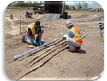
Field staff used direct push technology (DPT) to evaluate chlorinated solvent mass partitioning at finite intervals in the subsurface.
